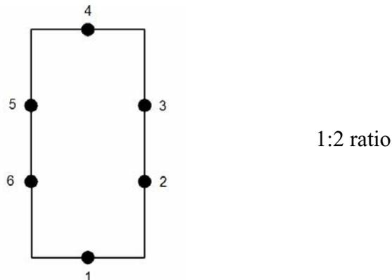
Figure 4. Boundary discretization using six constant boundary elements.
