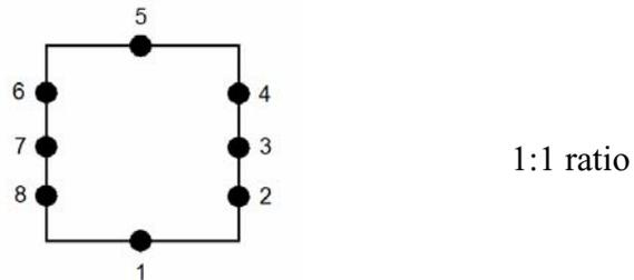
Figure 7. Boundary discretization using eight constant boundary elements.
