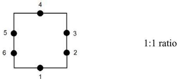
Figure 6. Boundary discretization using six constant boundary elements.
