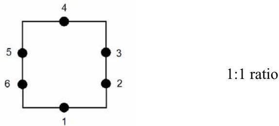
Figure 3. Boundary discretization using six constant boundary elements.
